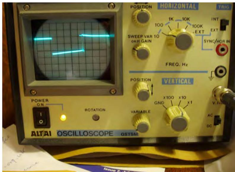
Above picture shows sharp rise & fall of square wave edges, measured at the lamp bulb terminals. The scope happened to be set to "AC input", but the picture below was set to "DC input" and shows a squarer square wave. The vertical DC voltage difference between the two lines below, is 1.5 volts:
