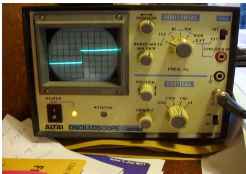
The picture below shows the waveform at either side of the  $0.56 \mu\text{F}$  capacitor (on flasher circuit board), showing a sharp rise but a ragged fall. However, the final result across the lamp terminals is all that is necessary (the picture above).
