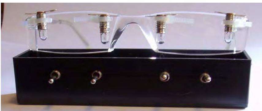
Four 6-volt 'Lilliput' bulbs are secured to 'ReadySpex' plastic spectacles, with 4 cable ties threaded through 8 holes drilled through the plastic lenses. (Shown resting on the switchbox with a switch for each bulb.)
